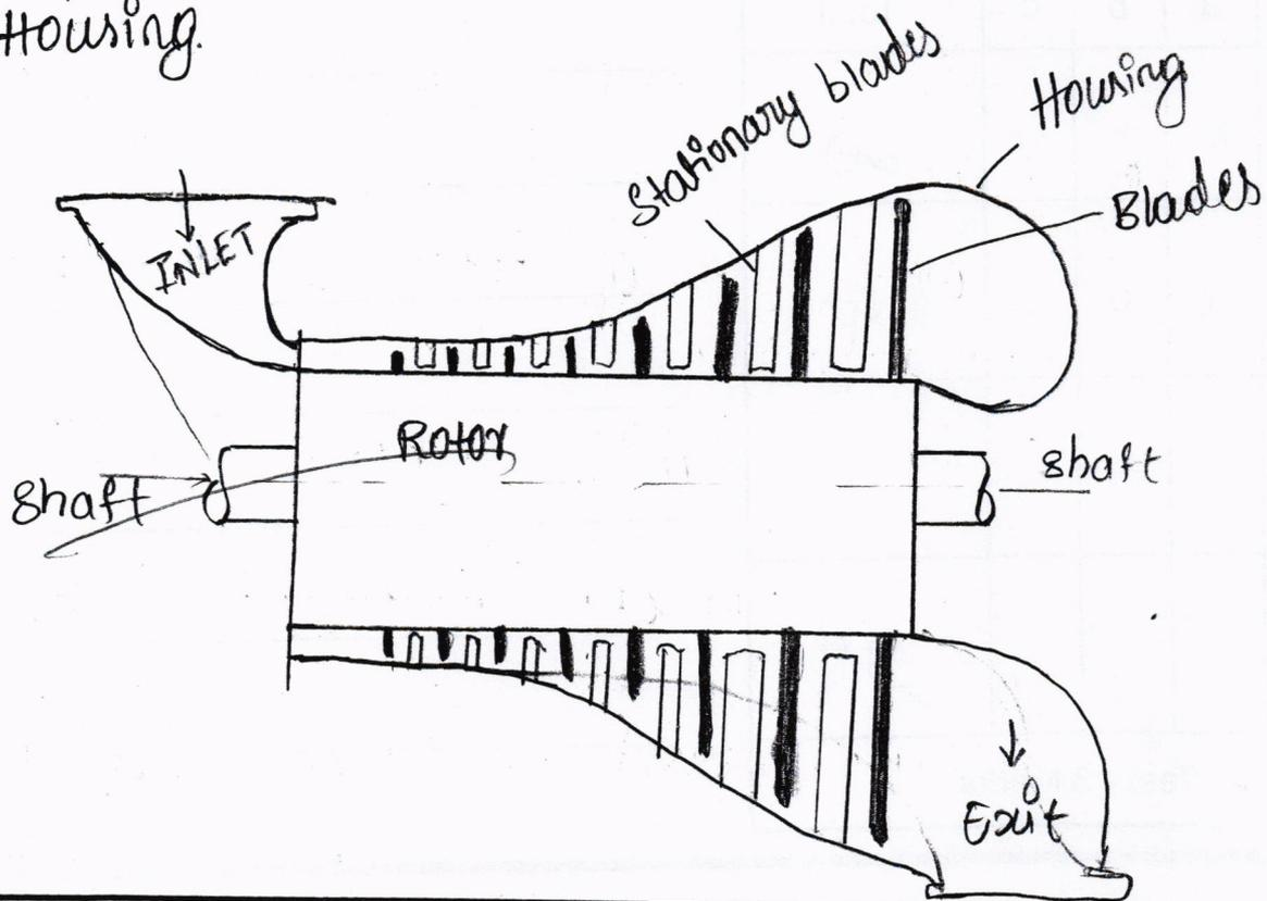
1. Rotating element :- Rotating elements are rotor, runner, impeller depending upon the type of flow. Energy transfer takes place b/w flowing fluid & a rotating element and results in the momentum change.
