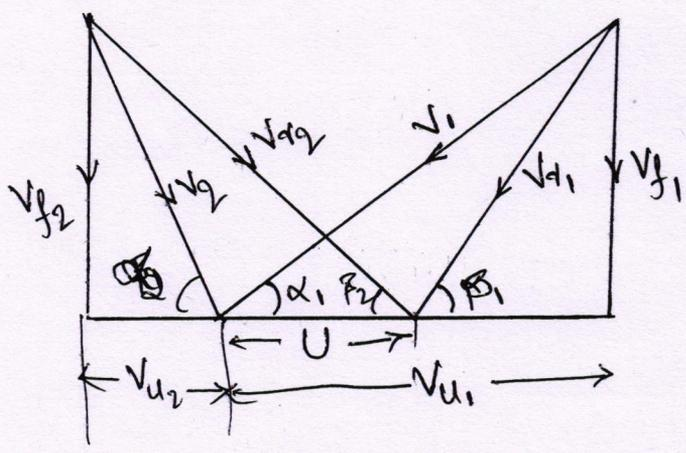
$$U = \frac{\pi DN}{60} = \frac{\pi \times 0.75 \times 3500}{60} = \underline{\underline{137.45 \text{ m/s}}}$$
