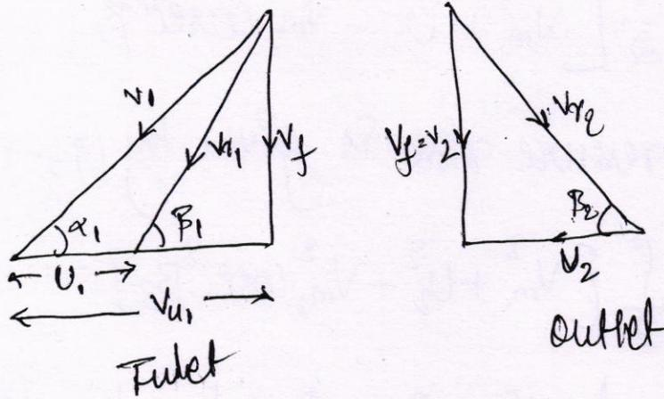
Francis turbine is an inward flow, medium head reaction turbine. Molecular Francis turbines are mixed flow type, in which water enters the runner radially & leaves axially at the center.
