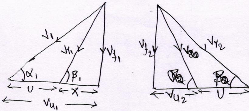
From fig.  $\sin \alpha_1 = \frac{V_{f1}}{V_1}$
